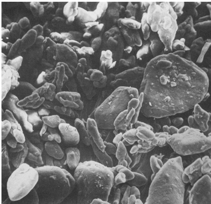
Fig. 3. SEM of paracetamol microcapsules containing solidified spheroid droplets of Eudragit RS polymer. Magnification 130:1.
