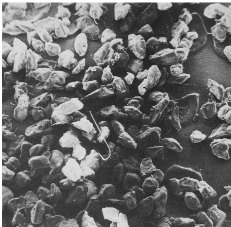
Fig. 1. SEM of paracetamol microcapsules coated with Eudragit RS polymer. Magnification 25:1.
